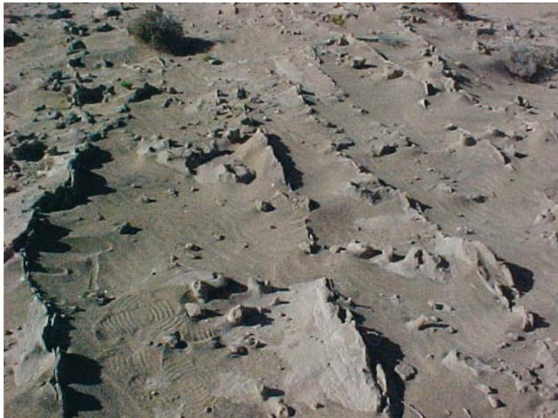
*Figure 8.* Clastic dikes in the area of greatest density of liquefaction features. For scale purposes the dikes' height is between 5 and 10 cm, and their length is tens of meters.
