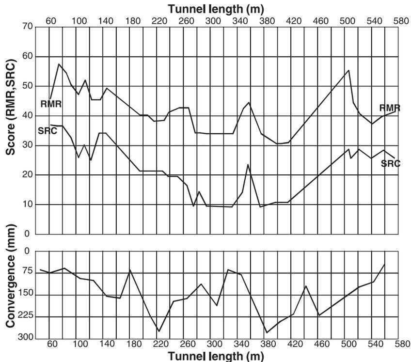
Fig. 4. RMR and SRC indices and convergence values for the Val Lemme Tunnel, a tunnel with a thin overburden and schistosity parallel to the tunnel axis (Bellini, 1998).
