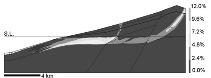
Figure 4. Shear strains using pressuremeter moduli for hyaloclastites (maximum shear strain 11.24%). Same scale horizontal and vertical.
