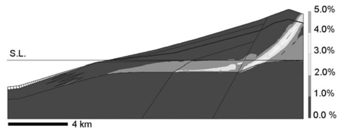
Figure 3. Shear strains using Table 2 properties (maximum shear strain 4.3%). Same scale horizontal and vertical.
