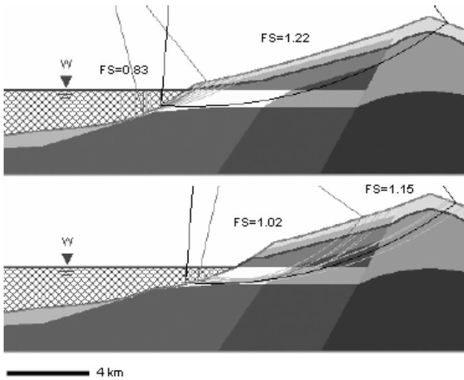
Figure 5. Limit equilibrium analysis results showing potential failure surfaces for the properties included in Table 1 and considering  $c = 0.1$  MPa and  $\phi = 14^\circ$  for hyaloclastites. Same scale horizontal and vertical.
